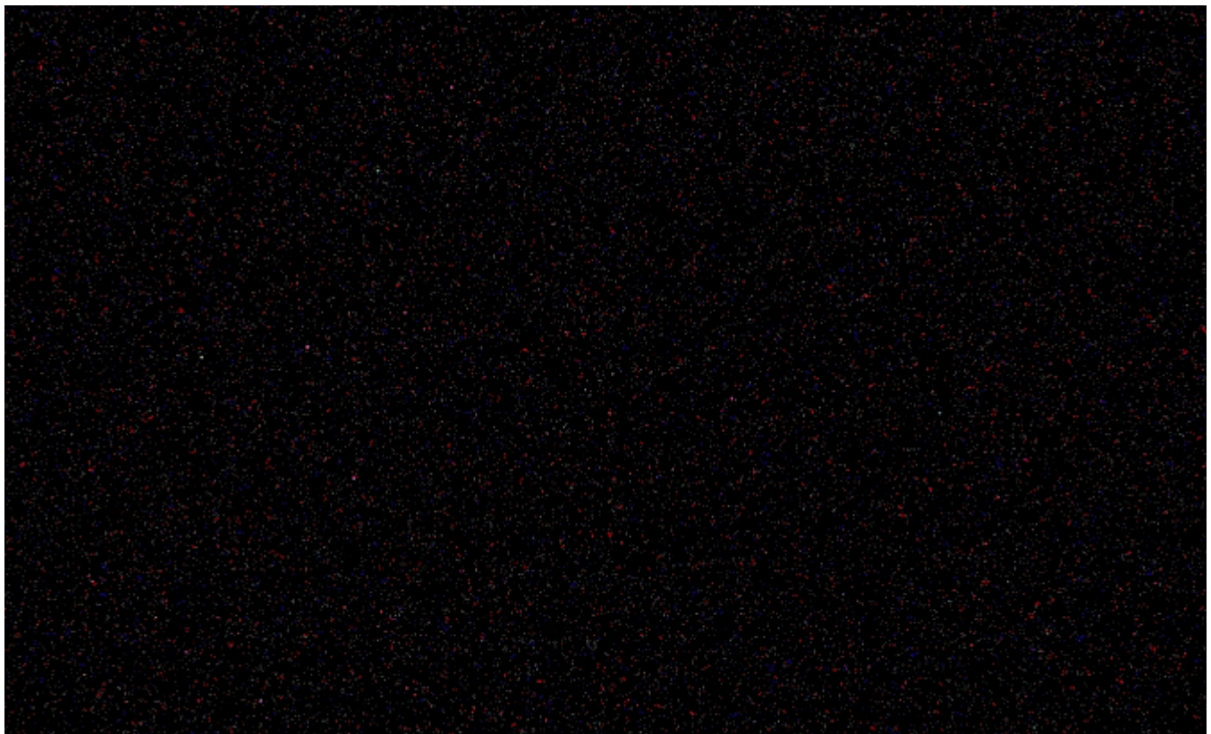
Above, Figure 2: Dark frame 20 minute exposure using a Canon 40DH. The center part, 1400 by 850 pixels, of the image is shown above. Temperature was 70°F
